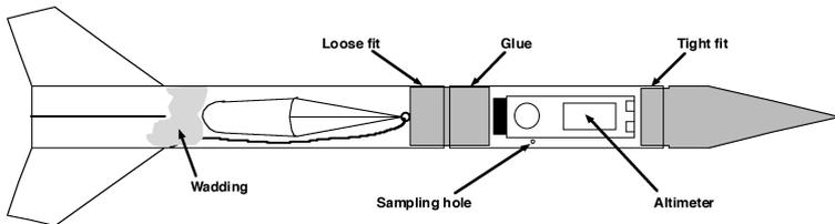
Perform initial testing of your rocket without the altimeter installed. Make sure that the parachute is ejected and opens properly so that you have a slow and safe landing. If you
