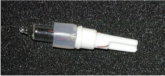
Silicone tube in place.
