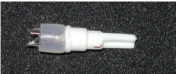
Bulb tip snapped off, filament exposed.
