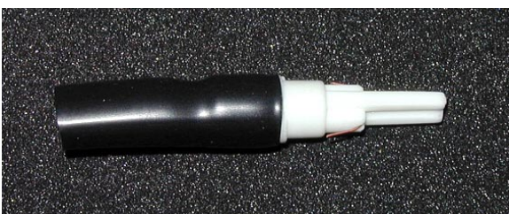
Heat shrink tube installed and shrunk.
