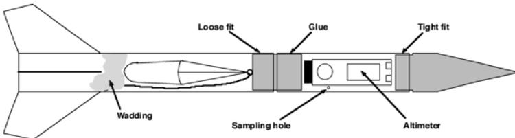
Perform initial testing of your rocket without the altimeter installed. Make sure that the parachute is ejected and opens properly so that you have a slow and safe landing. If you conduct your preliminary tests with the altimeter installed and the chute doesn't eject, the resulting high speed ballistic descent could damage the altimeter (in addition to your rocket!).
