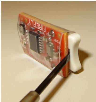
*To remove battery, pry the battery tray out with a small screwdriver (see description on preceding page).*
