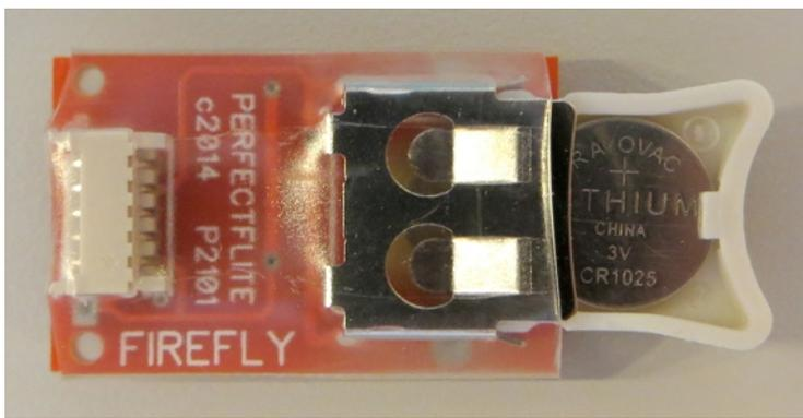
*Install battery with "+" terminal (big end) up.*
