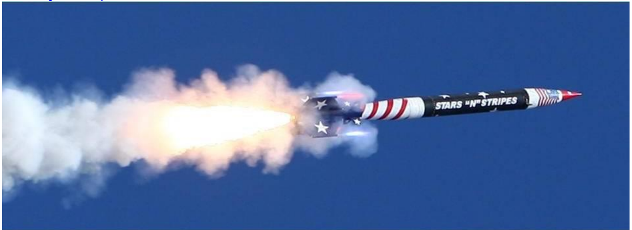
Figure 8. The 17' Tall Stars "N" Stripes Rocket Fires 4 Red and Blue H-Class Retro-Rockets to fight against the White N-Class Main Engine in Order to Limit Altitude (Photo Credit Ray LaPanse)
