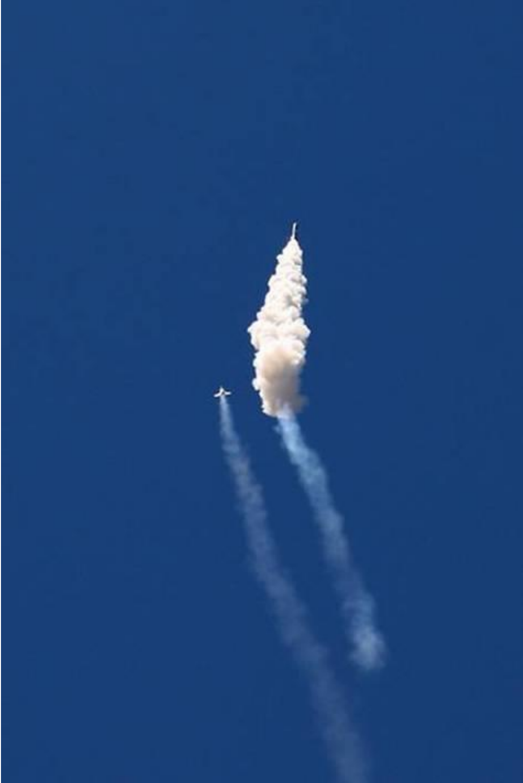
Figure 12. Future 1 st Stage Separation and 2 nd Stage Ignition. (Photo Credit Ray LaPanse)
