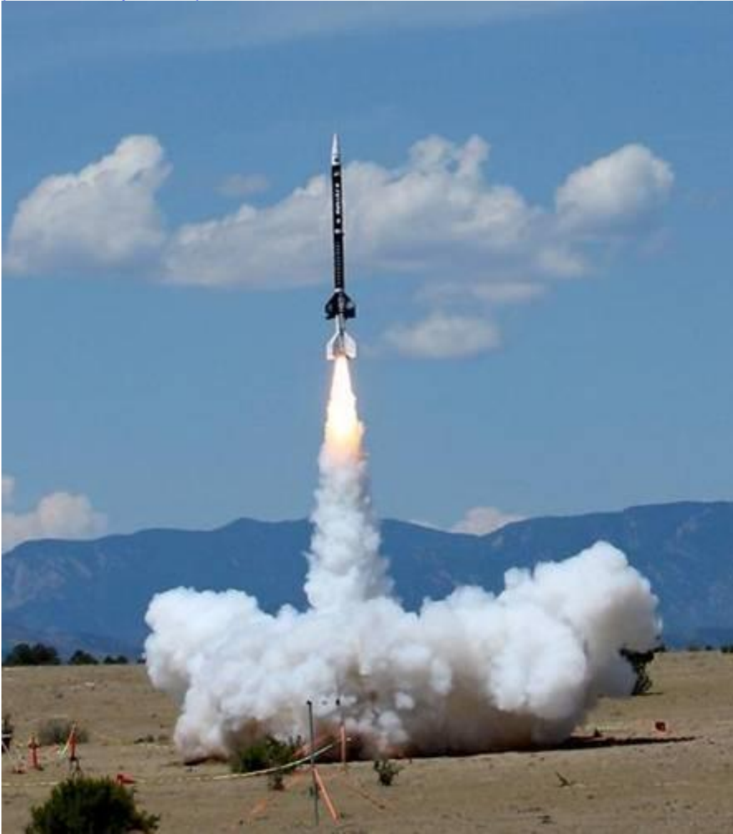
Figure 11. Liftoff of the 25' Tall Future Rocket Powered by Twin N2000W 1 st Stage Engines (Photo Credit Ray LaPanse)
