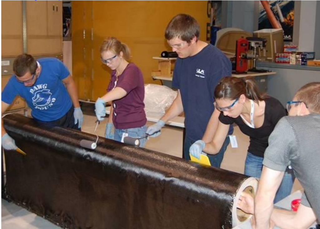
Figure 4. Interns Handcrafting the Carbon Fiber Airframe for the 2011 Future Rocket (Photo Credit Greg Arend)
